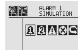
Figure 16. Alarm/Fault Simulation Menu
