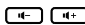
In idle mode or during ringing: increase or decrease ringer volume In communication: increase or decrease handset or hands-free volume
