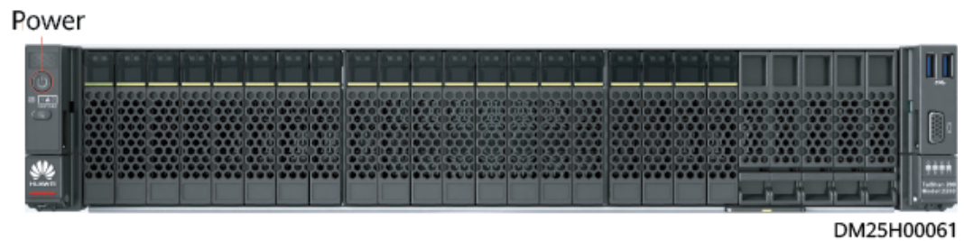
Figure 7-34 TaiShan 200 server power button
