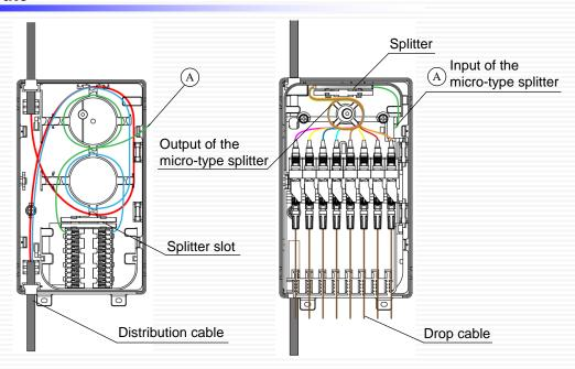
Type1: with 900µm pigtail type splitter
