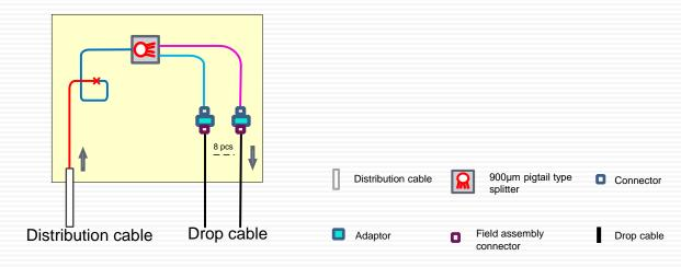
Type 2: In line type or mid-span type
