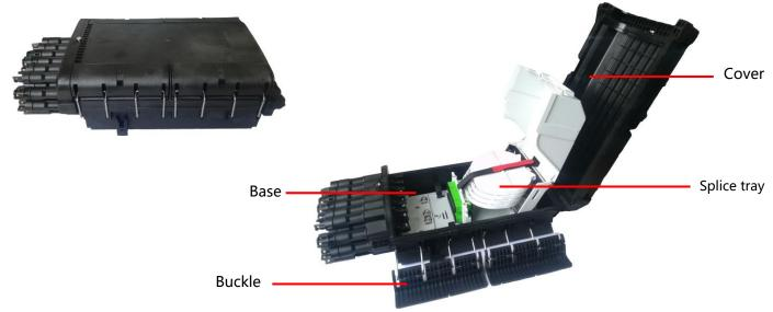
FDP-430D boxes can be used as fiber distribution box or fiber access terminal box. It is designed to install in burial or duct environment which can keep internal components away from outdoor environmental damage and provide a protected access point. The distribution fiber is spliced to the input of the optical splitter. The splitter outputs are terminated/splice to connect with drop cable.
