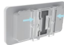
Removed by pushing inwards on both sides
