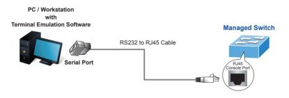
Figure 4-1 Managed Switch Console Connectivity
