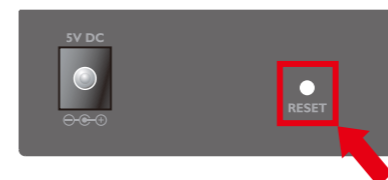
Figure 7-1: ICS-110/ICS-115A Hardware-based Reset Button
