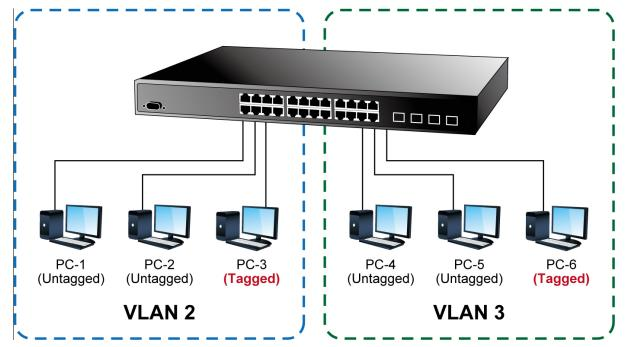
Figure 4-6-8: Two Separate VLAN Diagram
