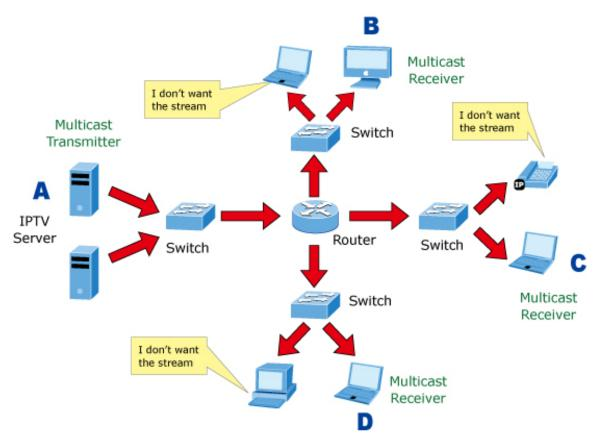
Figure 4-8-2: Multicast Flooding
