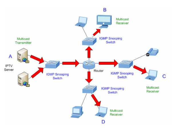
Figure 4-8-3: IGMP Snooping Multicast Stream Control
