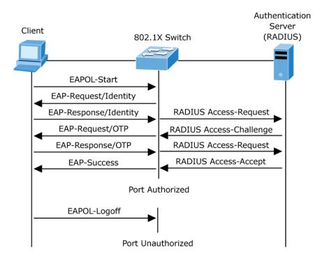
Figure 4-11-2: EAP Message Exchange
