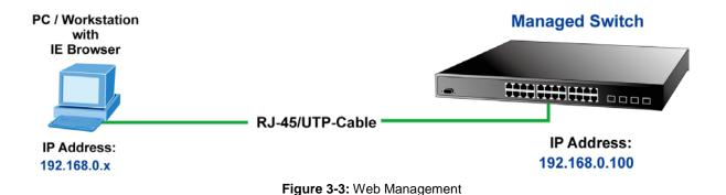
You can then use your Web browser to list and manage the Managed Switch configuration parameters from one central location, just as if you were directly connected to the Managed Switch's console port. Web Management requires either **Microsoft**Internet Explorer 7.0 or later, Safari or Mozilla Firefox 1.5 or later.
