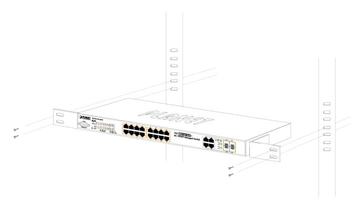
Figure 2-6: Mounting Managed Switch in a Rack
