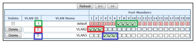
Figure 4-6-9: Add New VLAN Group, assign VLAN Members for VLAN 2 and VLAN 3 and Remove Specify Ports from VLAN 1
