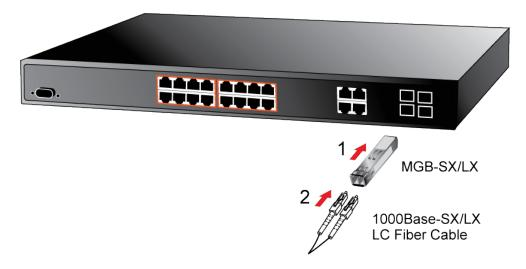
Figure 2-7: Plug-in the SFP Transceiver
