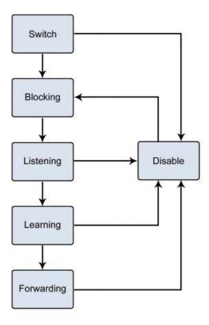
Figure 4-7-1: STP Port State Transitions
