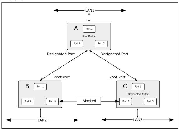
Figure 4-7-3: After Applying the STA Rules
