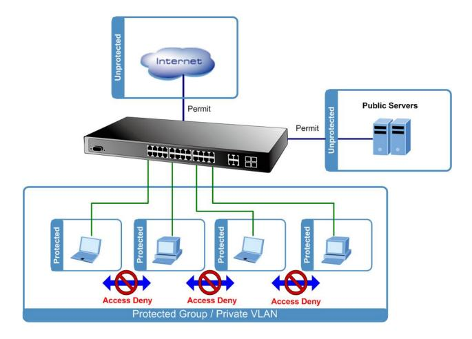
For private VLANs to be applied, the switch must first be configured for standard VLAN operation When this is in place, one or more of the configured VLANs can be configured as private VLANs. Ports in a private VLAN fall into one of these two groups:
