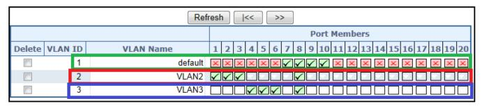
Figure 4-6-12: VLAN Overlap Port Setting & VLAN 1 – The Public Area Member Assign
