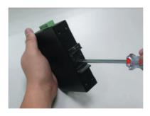
Step 1: Screw the DIN-rail on the Industrial Gigabit Media Converter.
