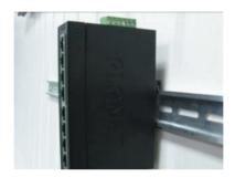
$\textbf{Step 3:} \quad \text{Make sure the DIN-rail is tightly secured on the track.}$
