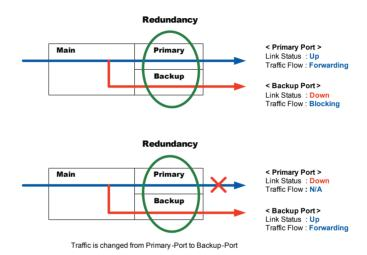
Figure 3-3: Redundancy Behavior Topology
