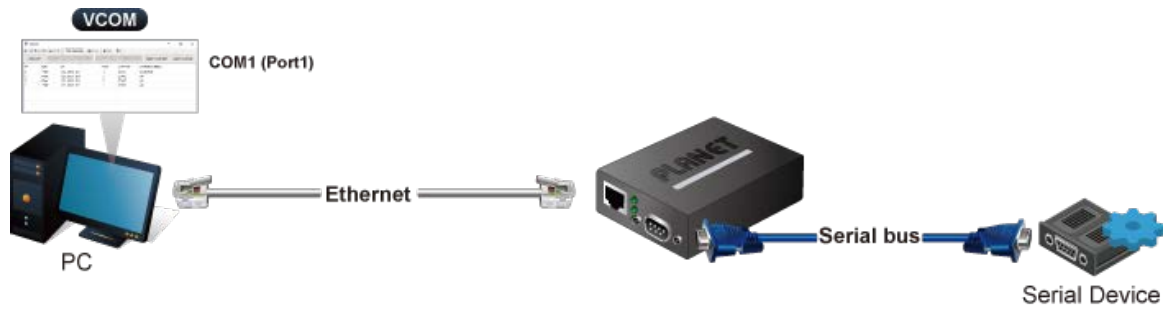
Figure 4-5-26: Virtual COM Mode Topology
