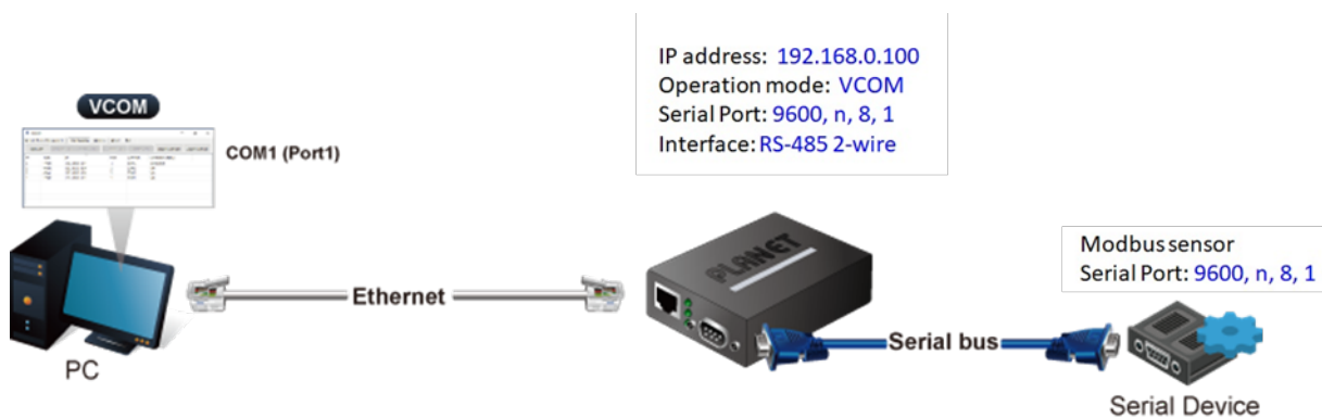
Figure 4-5-28: Virtual COM Mode Application
