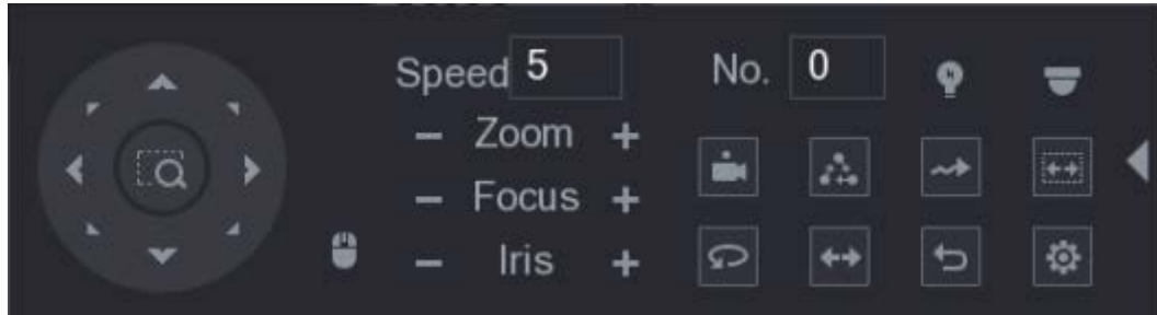
Figure 5-63 Panel de control PTZ ampliado
