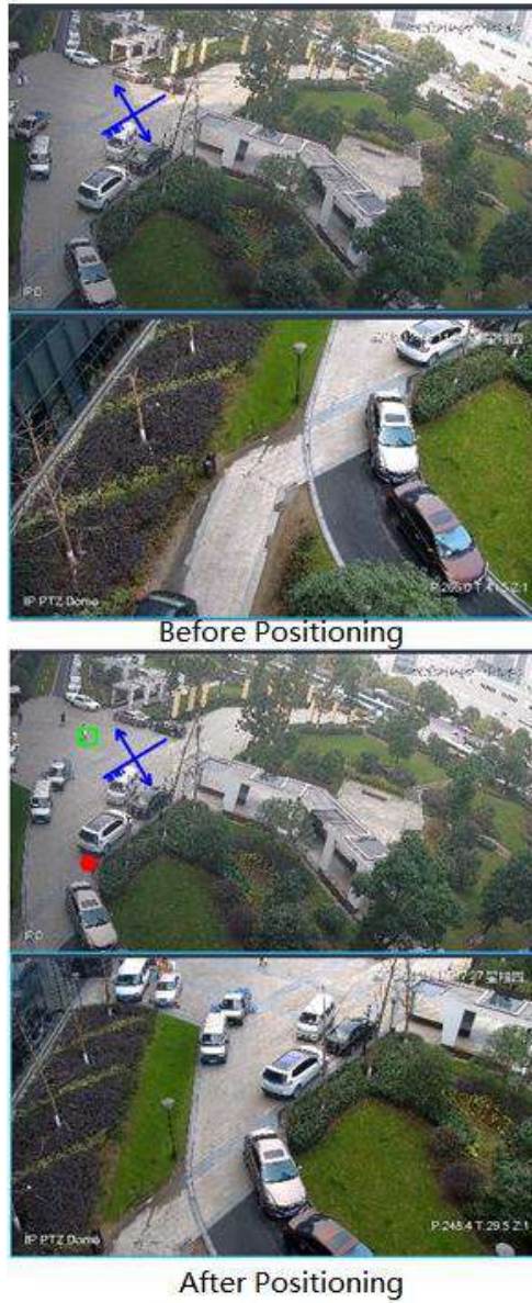
Figure 5-49 3D positioning (Zoom in after positioning)
