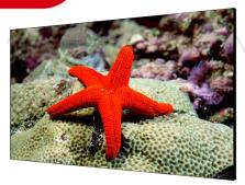
The DS-D2055LU-Y LCD display uses an industry-level ultra-narrow bezel design, which enables a bezel width of 3.5 mm between neighboring displays. The adopted direct-lit LED backlighting technology helps achieve ultra-high and uniform brightness of 500 cd/m² without boundary shadows. The display has abundant interfaces for video inputs, such as DVI, VGA, HDMI, and DP.
