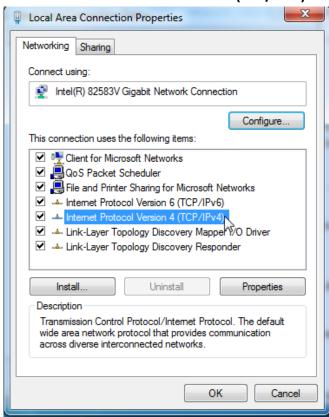
5) Select **Use the following IP address**, set the **IP address** to **192.168.1.***X* (*X* ranges from 2 to 253, excluding 35 and 36), the **Subnet mask** to **255.255.25.0**, and click **OK**.
