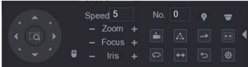
Figure 5-63 Panel de control PTZ ampliado
