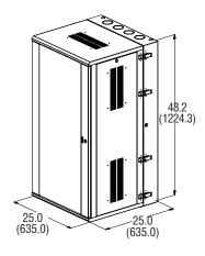
PZWMC12W - Wall Mount Cabinet with windowed door PZWMC18W - Wall Mount Cabinet with windowed door
