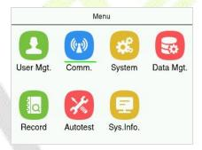
**2.** Then click **Comm.** > **Wi-Fi setting** to enter the Wi-Fi setting interface. And the device will search for available Wi-Fi within the network range.
