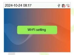
1. Pressing **M/OK** in this shortcut interface will directly enter the Wi-Fi setting interface. The device will search for available Wi-Fi networks within range.
