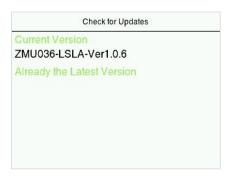
If the firmware version of the device is not the latest, the version number and change log of the latest version will be displayed. Users can choose whether to update to the latest firmware version.
