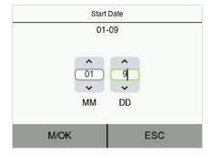
When restoring the factory settings, the time (24-hour) and date format (YYYY-MM-DD) can be restored, but the device date and time cannot be restored.
