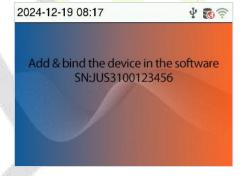
**Note:** If you are using the device for the first time or if the device is not bound, the Wi-Fi shortcut interface will take you directly to the SN interface after you set up Wi-Fi. In this screen you can view the serial number of the device.
