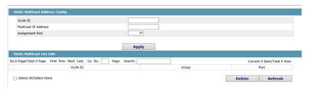
This page displays the static multicast group in current network according to IGMP-Snooping statistics and the port set each member belongs to.
