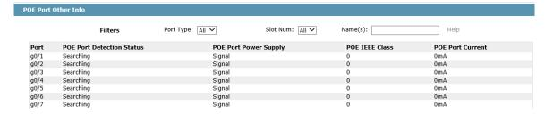
On this page, you can check POE Port Detection Status, POE Port Power Supply, POE IEEE Class, and POE Port Current.
