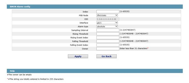
The index is used to identify a specific alarm information; if the index is same to the previously applied index, it will replace the previous one.
