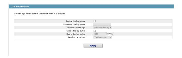
If "Enabling the log server" is selected, the device will transmit the log information to the designated server. In this case, you need enter the address of the server in the "Address of the system log server" textbox and select the log's grade in the "Grade of the system log information" dropdown box.
