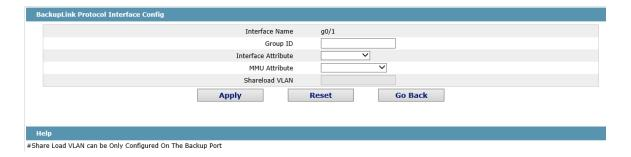
The backup link group which has configured the primary port cannot take other ports as its primary port. Likewise, the backup link group which has configured the backup port cannot take other ports as its backup port.
