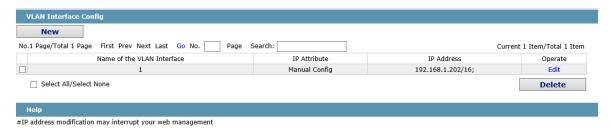
Click **New** to add a new VLAN interface. Click Cancel to delete a VLAN interface. Click Modify to modify the settings of a corresponding VLAN interface.
