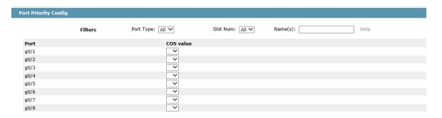
You can set the CoS value by clicking the dropdown box on the right of each port and selecting a value. The default CoS value of a port is 0, meaning the lowest priority. If the CoS value is 7, it means that the priority is the highest.
