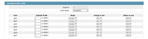
If you want to create a new VLAN, enter a VLAN ID and a VLAN name; the VLAN name can be null.
