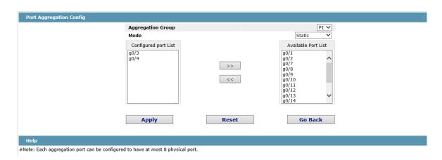
An aggregation group is selectable when it is created but is not selectable when it is modified.
