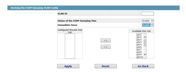
When create new IGMP-Snooping Vlan, VLAN ID can be modified; when modify IGMP-Snooping Vlan, VLAN ID cannot be modified.
