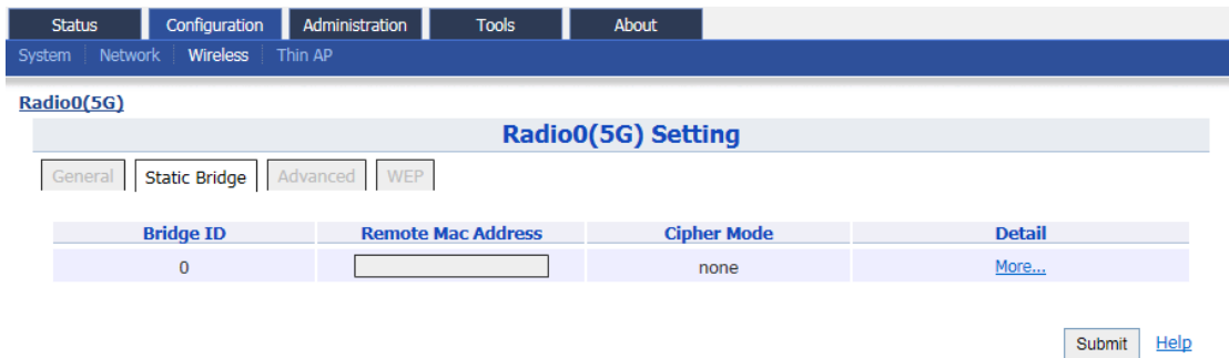
Figure 5-51 5G bridge setting
