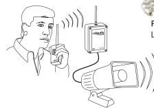
Note: For proper operation the LoudMouth radio receiver and 2-way radio must operate on the same frequency and tone. For selective paging capability 2-way radio must be capable of 2-tone encoding.
