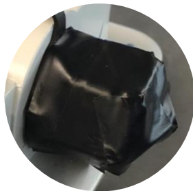
Wrap a layer of electrical tape all over the Ethernet port
