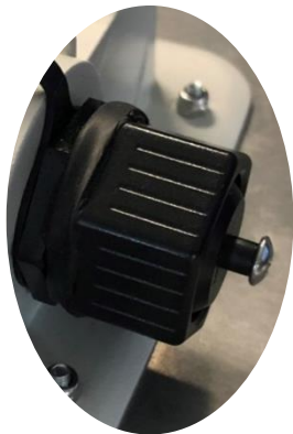
Tighten Ethernet Cap Nut with Rubber Mastic Tape around
