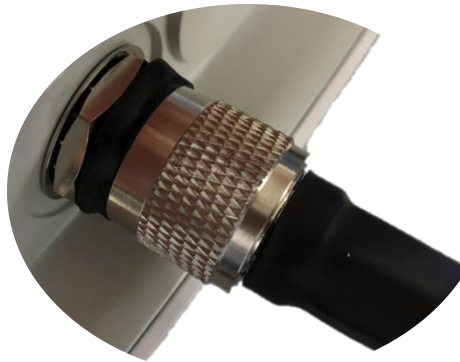
Figure 10-12 Tighten the RF Cable/Antenna Connectors around the Antenna ports
