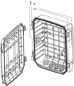
Pass the Ethernet and I/O combo cables through the M20 cable glands, and into the cabinet. You may }^^åk[أ[]^}k@^\&aài}^¢k\ù^&`|^\&@{\ak}&{\cish.e.[] } bk[\\ the cabinet. You can then install the camera. Refer the camera's documentation for information.
