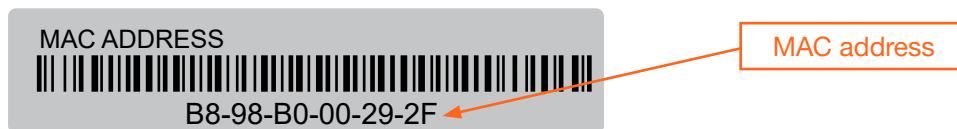
Figure 1.1 - Sample MAC address label found on the side of an AT-ANC-108D.
