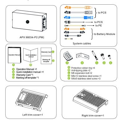
Figure 4-5: Components of the APX 98034-P2
