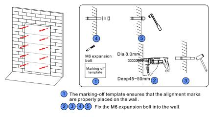
Figure 4-16: The marking-off template and install the expansion bolt
