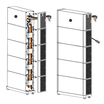
Figure 4-26: Installing external cables
