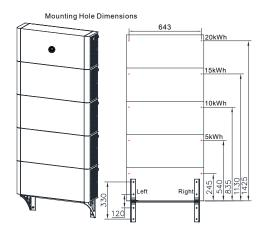
Figure 4-7: Mounting Hole Dimensions
