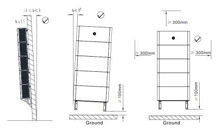
Figure 4-1: Wall-mounted installation
