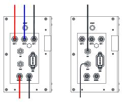
Figure 4-24: APX 98034-P2 wiring diagram
