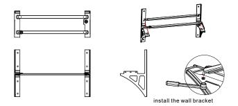
Figure 4-8: Install the mounting bracket
