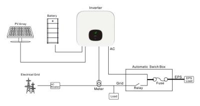
Figure 1-1: System diagram of APX High voltage battery system
