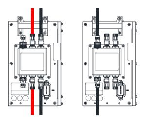
Figure 4-25: APX 5.0P-B1 wiring diagram
