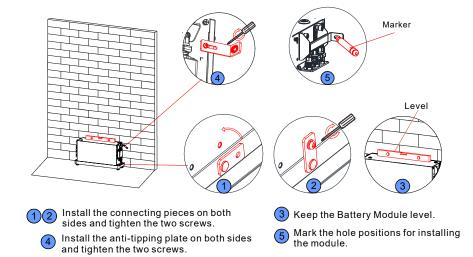
Figure 4-15: Installing the battery support
