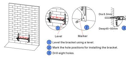
Figure 4-9: Determine the hole positions for installing the bracket
