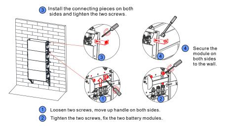
Figure 4-12: Install the battery module
