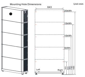
Figure 4-14: Mounting Hole Dimensions
