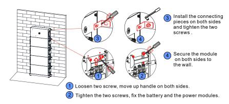
Figure 4-18: Install the power module
