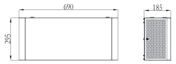
Figure 1-6: Dimensions of APX 5.0P-B1
