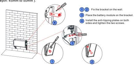
Figure 4-10: Fix the bracket to the wall
