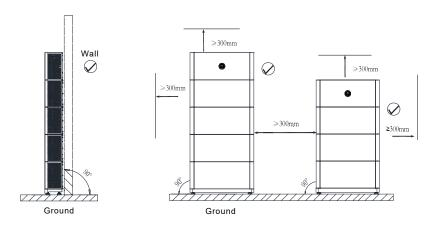
Figure 4-2: Floor-mounted installation
