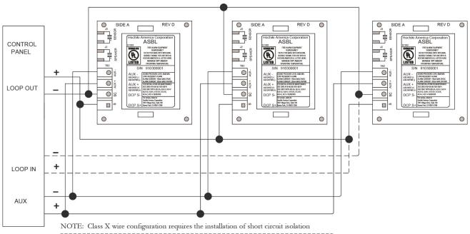
DO NOT CONNECT FOR CLASS B CONNECT FOR CLASS X
