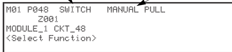
Figure 9-6 Programming Points as Inputs for the 5880 Module
