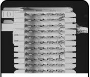
Route each pair through the same slot in the fanning strip in its mated state. Separate the conductors of each pair inside the fanning strip and place in the appropriate quick clips. Pair twist must be maintained to within .05 in. of the point of termination for category 5e installations. Check the conductor sequence at this point and correct any miswires or reversals.
