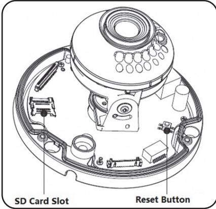
**Note:** For reset (used to return the camera settings to factory default mode), long press for 10 seconds and then the light turns off.
