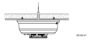
Figure 3. Mount Detector Across Ceiling Panel Support
