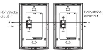
Signal polarity shown in the active condition.
