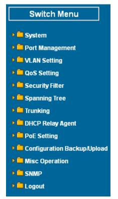
Figure 4-1-2 PoE Web Smart Switch Main Functions Menu
