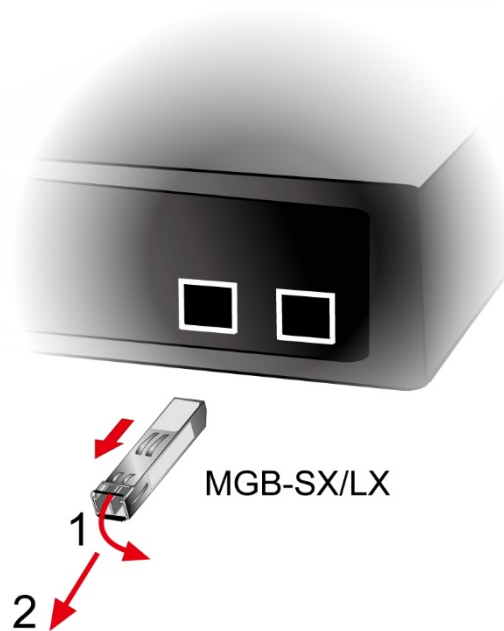
Figure 2-2-5: How to Pull Out the SFP/SFP+ Transceiver
