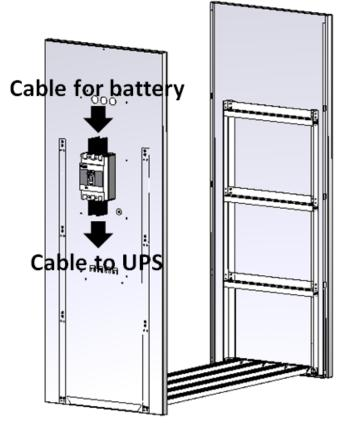
Step3. Install the snap bushing\*3pcs (Note: User can cut the snap bushing to insert the cable) and paste the label on the rear panel then fixed the screw (M5\*1pcs) on the ground(It is for ground connection).
