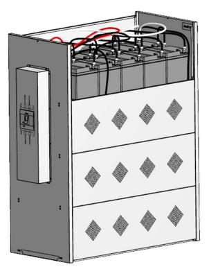
Step 10. Put on the top panel and tighten the screw(M3 screw\*1pcs). Please let the cables connect with breaker when you want to connect battery cabinet from UPS.
