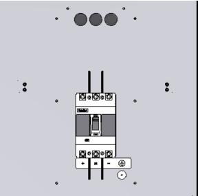
Step 4. Put the batteries on the bracket and connect the cables (let the terminals had a little angle that could easy to install).
