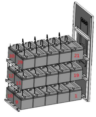
Step 7. Install the fourth bracket and put the batteries then connect the cables (Battery\*10pcs/L2\*5pcs/L3\*4pcs/L6\*1pcs/L7\*1pcs)
