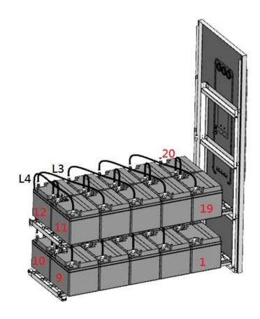
Step 6. Install the third bracket and put the batteries then connect the cables (Battery\*10pcs/ L2\*5pcs/L3\*4pcs/L1\*1pcs)
