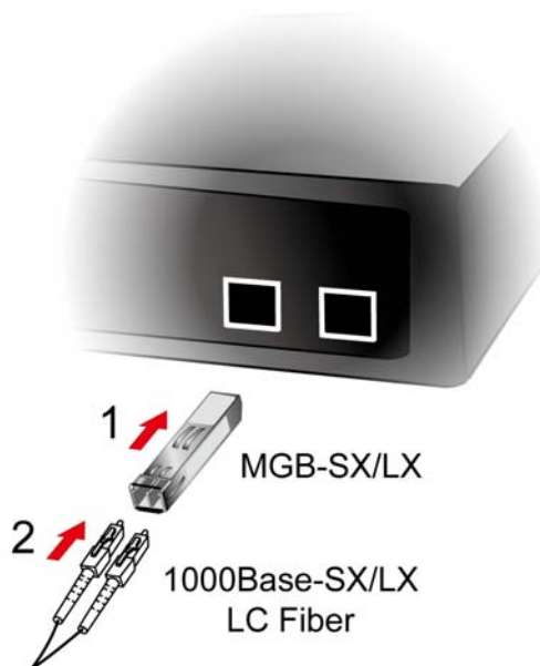
Figure 2-7 Plug in the SFP transceiver
