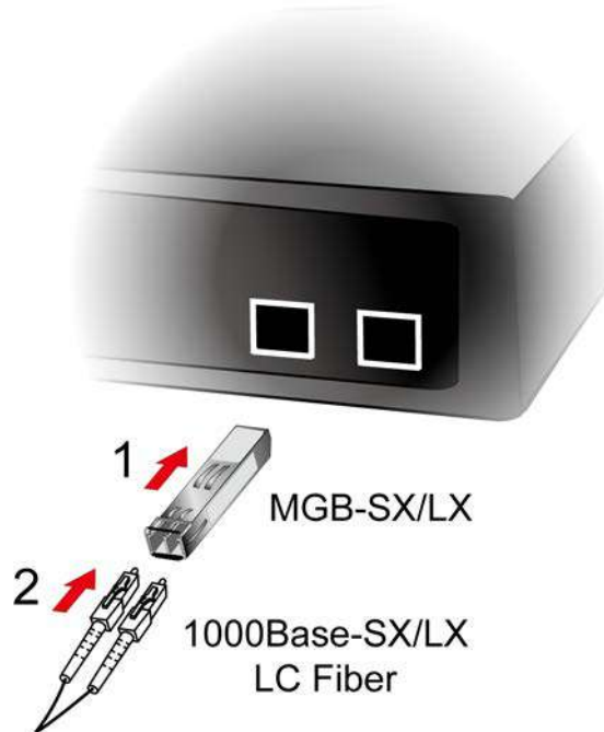
Figure 2-2-4: Plug-in the SFP/SFP+ Transceiver
