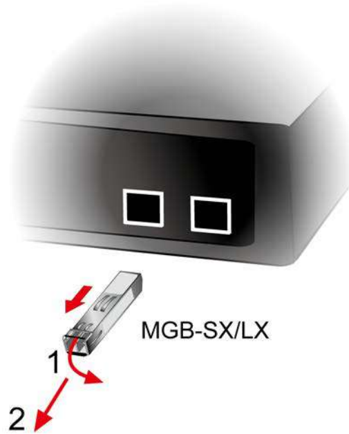
Figure 2-2-5: How to Pull Out the SFP/SFP+ Transceiver
