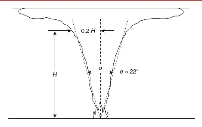
NFPA 72 2016 - B.4.9.1 The Plume Divergence of an Unconstrained Fire
