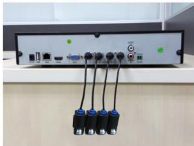
Baluns click together for a neat installation
