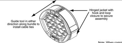
Note: When complete slide reusable tool off of cable bundle
