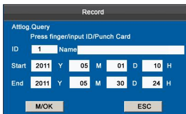
Press finger/input ID/Punch Card, enter the Start and End using keypad, then press OK .
