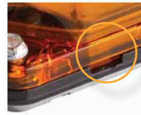
For ease of service while on the vehicle, the dome can be removed from the base by simply removing (4) screws and lifting the dome in from one of the notches in the base.
