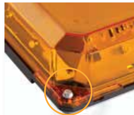
For ease of service while on the vehicle, the dome can be removed from the base by simply removing (4) screws and lifting the dome in from one of the notches in the base.
