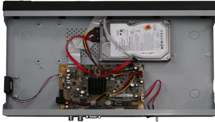
Figure 2. 9 Fix Hard Disk
