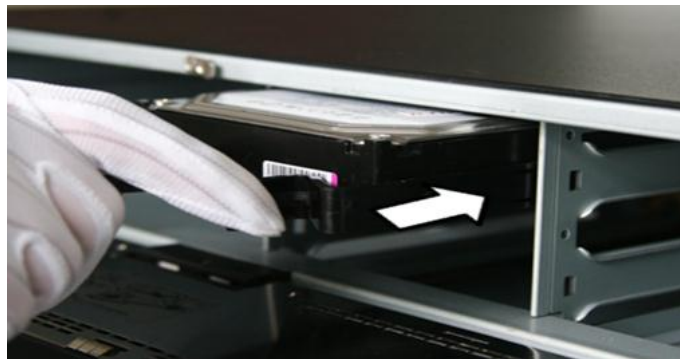
Figure 2. 4 Insert Hard Disk
