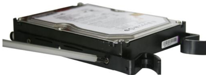
Figure 2. 1 Fasten Hard Disk
