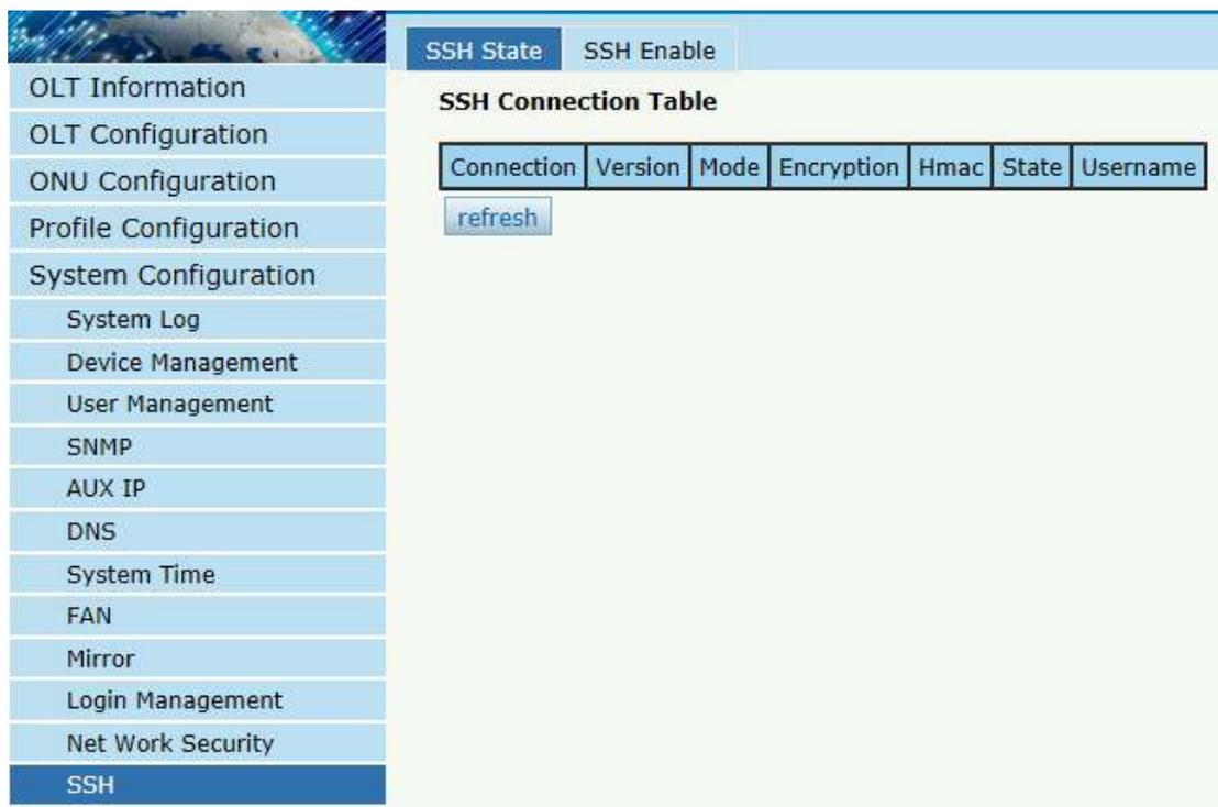
The screenshot displays the SSH configuration page. On the left, a navigation menu lists various system settings, with 'SSH' highlighted at the bottom. The main content area features a 'SSH State' indicator set to 'SSH Enable'. Below this is an 'SSH Connection Table' with columns for 'Connection', 'Version', 'Mode', 'Encryption', 'Hmac', 'State', and 'Username'. A 'refresh' button is located below the table header.
