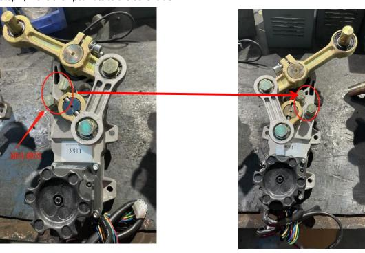
Step5, loose the screws of the balance rod
