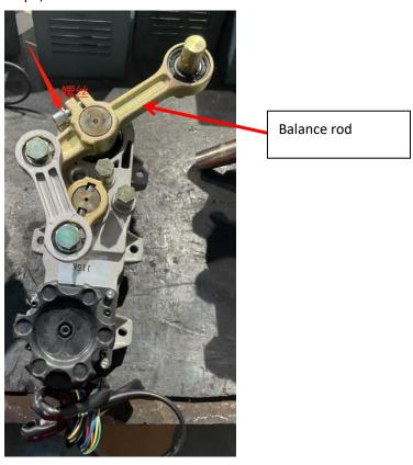
Step 6 Take off the balance rod and reassemble it by rotating the direction, and fix the mid-rod, make sure the boom holder is on vertical state, then tighten the screws.
