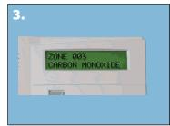
Verify CO sensing at the control panel. The detector will automatically exit RealTest alarm mode after about 20-60 seconds.
