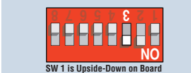
SW 1 is Upside-Down on Board SW 1, Switch 3 MUST be ON except for dual operators or exit loop partial open applications.
