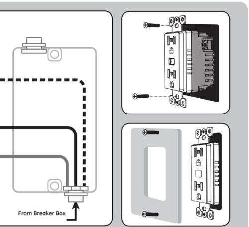
4. Reapply power to the circuit at fuse box or circuit breaker and test the system.
